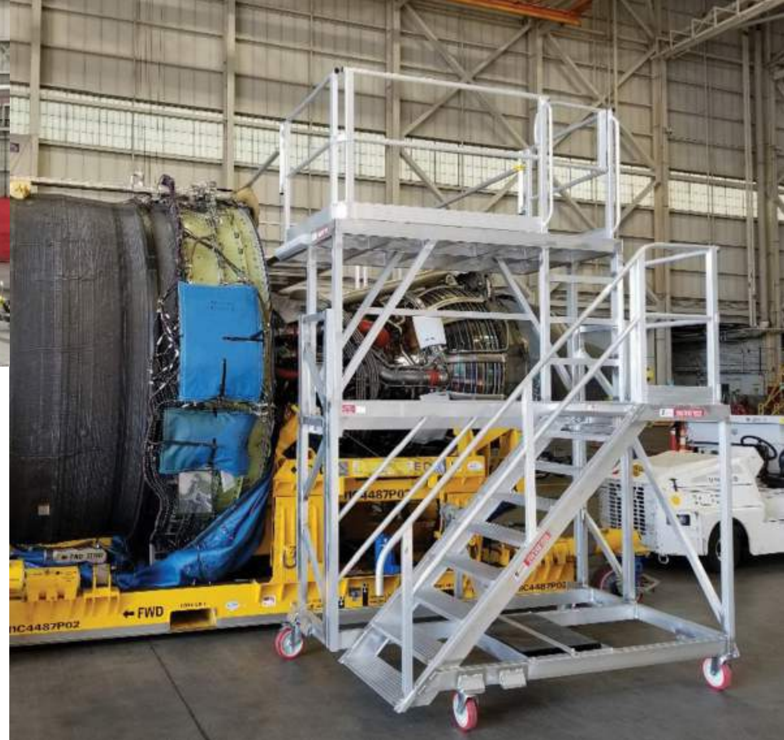
United's technicians can wheel two of SafeSmart's identically-mirrored arched access systems together to form one safe bridge over the aircraft's engines.
