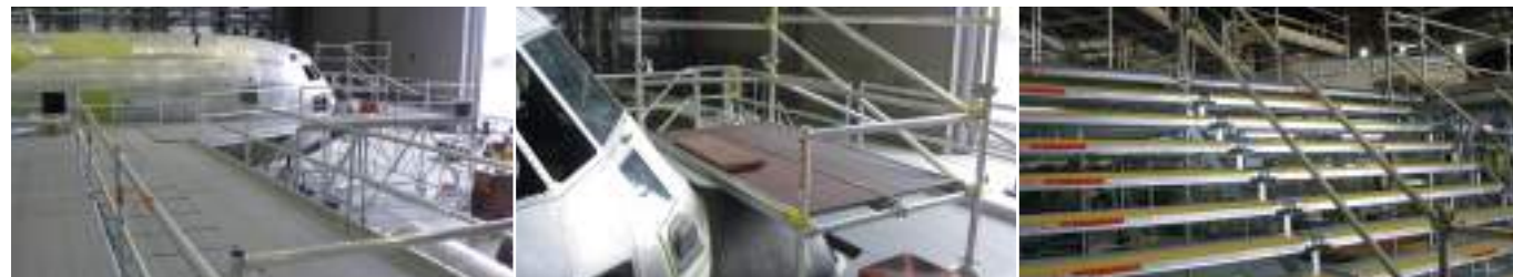
MOBILE SCAFFOLDING FOR WING PROTECTION DESIGNED TO AVOID USING HARNESES AND LANYARDS
